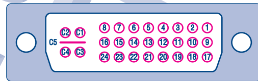
DVI-I digital cable Plug (viewed at pins)
